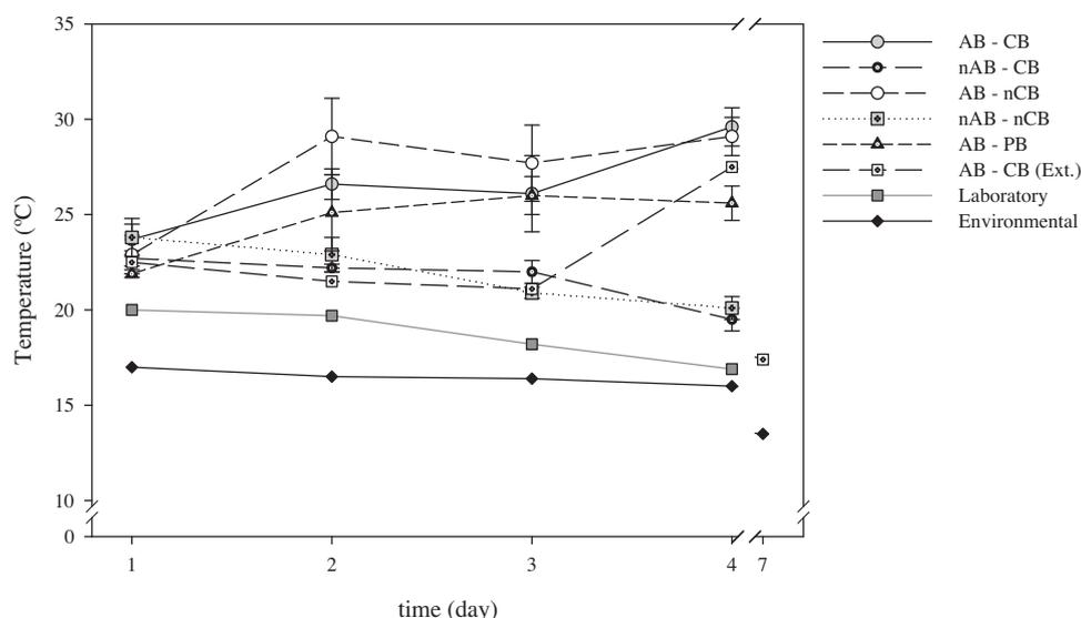
**Fig. 4.** Evolution of the temperatures measured inside each bin and around them (laboratory and environmental). AB-CB: aerated bin and compostable bag; AB-nCB: aerated bin and non-compostable bag; nAB-CB: non-aerated bin and compostable bag; nAB-nCB: non-aerated bin and non-compostable bag; AB-PB: aerated bin and paper bag. The results presented are the average of three experiments and the corresponding standard deviations.
